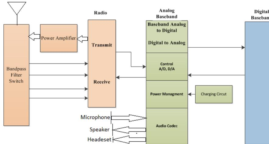
Figure 3. Functioning Diagram of Analog Base Band Processor
