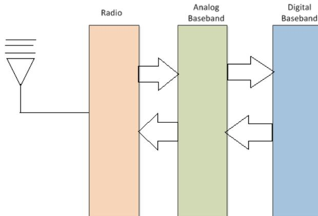
**Figure 1.**Block Diagram of GSM Modem components
