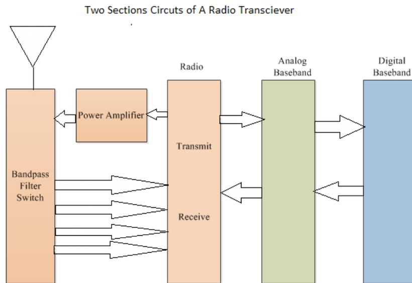
**Figure 2.** The Basic Operation Methods Of RF Section
