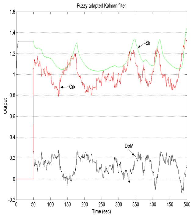
Figure 8. Fuzzy-adapted Kalman filter,  $Q$  fixed.
