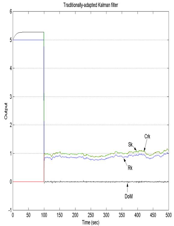
Figure 3. Traditionally-adapted Kalman filter, *Q* fixed.
