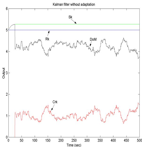
Figure 2. Kalman filter without adaptation, *Q* and *R* fixed.
