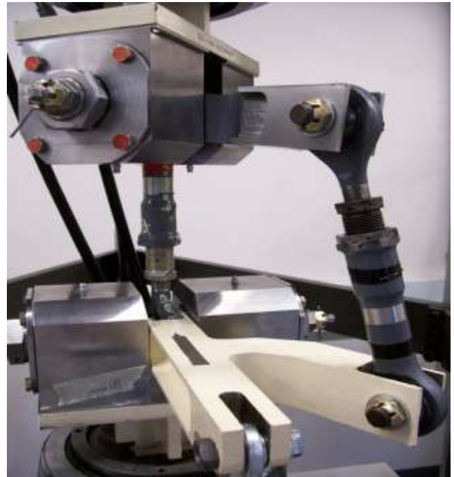
Fig. 3. A pair of pitch links undergoing laboratory wear testing to gather data for developing feature extraction algorithms. The link has a ball joint at each end which the WISD project aimed to monitor.
