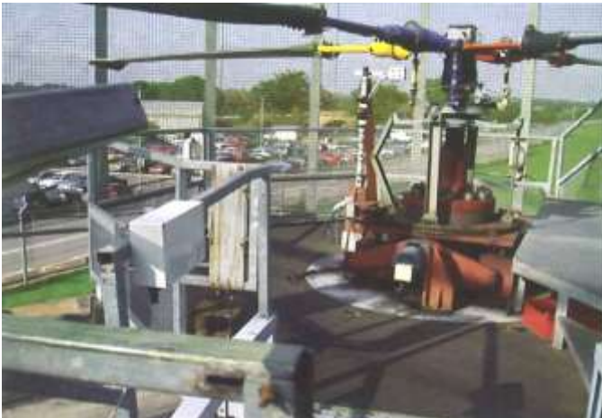
Fig. 9. Whirl tower installation with prototype WISD communication hardware installed.
