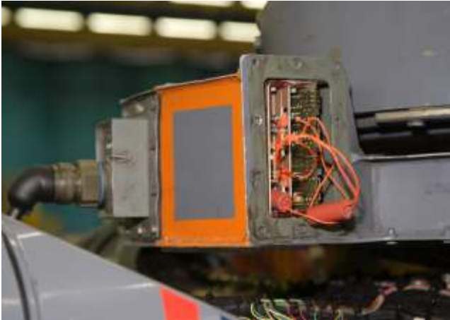
Fig. 12. Battery cards installed on the rotor head. The battery leads are shown unconnected prior to connection and final closure before flight.
