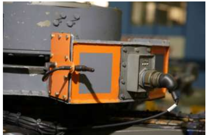
Fig. 11. WACD rotor mounted electronics. The orange painted box carries the signal conditioning, processing and communications electronics. The antenna is mounted on the tab nearest the camera.
