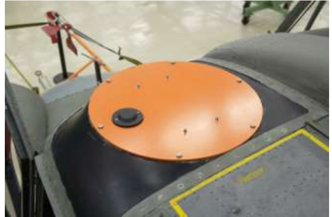
Fig. 14. Static airframe low profile antenna (black disk) mounted on the cockpit roof.
