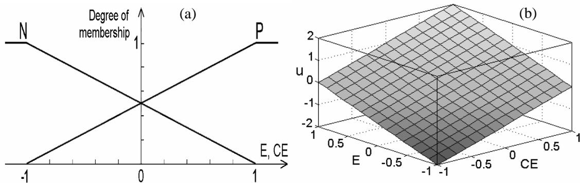
Figure 8.4 (a) Membership functions for  $E$  and  $CE$ ; (b) Control surface of the normalised and linear FCS.
