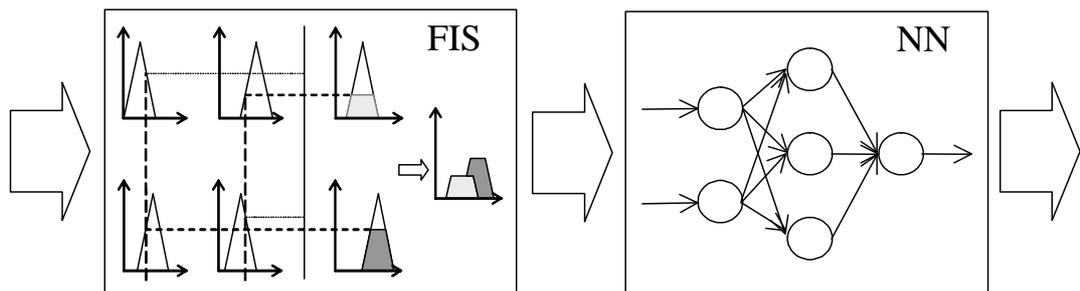
Figure 3.13 Concurrent neural/fuzzy system where a NN is used as a post-processor for a FIS.
