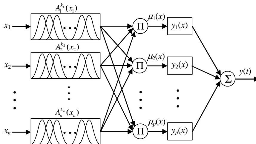
Figure 7.1 Graphical representation of the FIS defined by the rule base (7.5) and equation (7.7).
