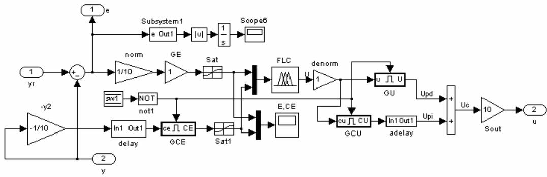
Figure B.30 Subsystem MHPID-FLC: MHPID-FLC and MSDF model.
