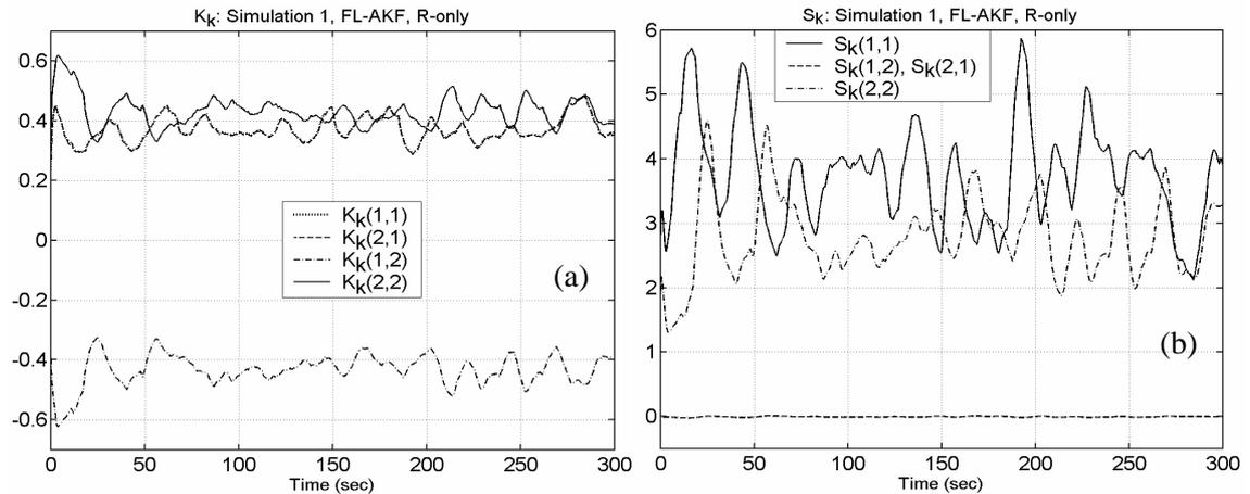
Figure 5.11(a) Elements of the Kalman gain matrix. (b) Elements of the residual covariance matrix; simulation 2, FL-AKF, R-only case.
