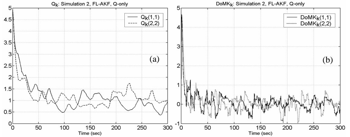
Figure 5.14(a) Estimated diagonal elements of the measurement noise covariance matrix  $Q_k$ . (b) Diagonal elements of matrix  $DoMK_k$ ; simulation 2, FL-AKF, Q-only case.
