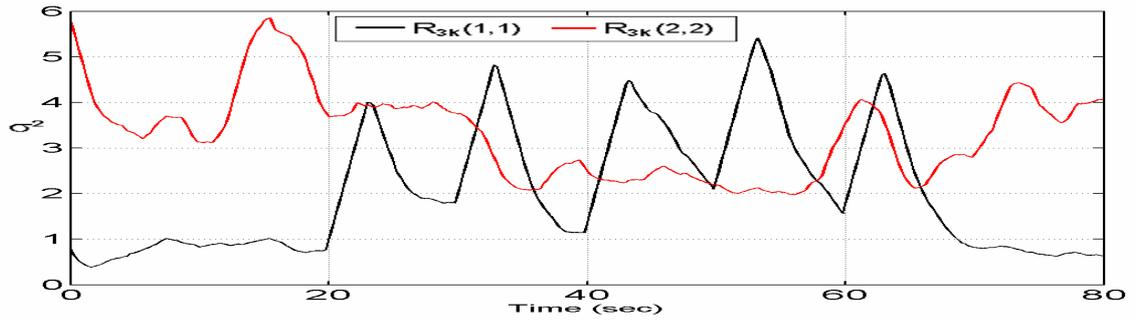
Figure 6.21 Adjustment of the elements in the main diagonal of matrix  $R_{3k}$ , FL-AKF 3, FL-AKF-FLA, simulation 6.
