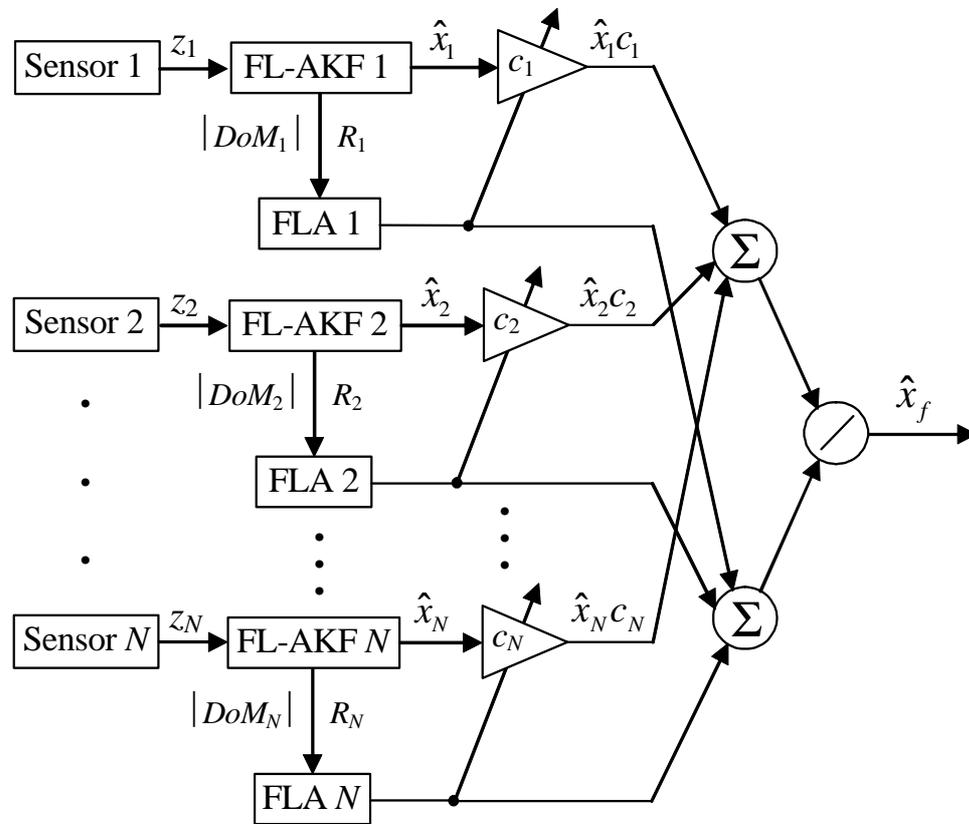
Figure 6.1 Proposed hybrid FL-AKF-FLA MSDF architecture (the time-step subscript is not indicated for simplicity).
