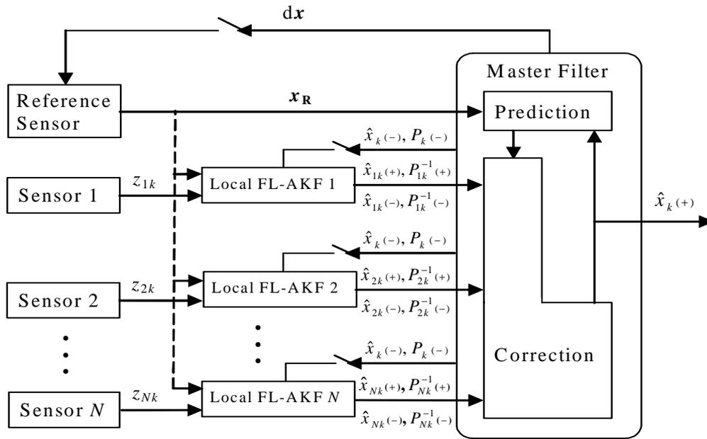
Figure 6.6 Fuzzy logic-based Adaptive Decentralised Kalman Filter (FL-ADKF).
