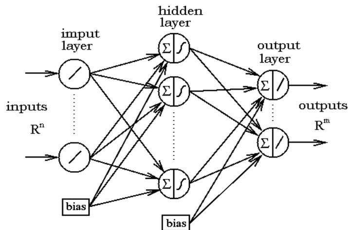
Figure 3.9 A typical feedforward NN.
