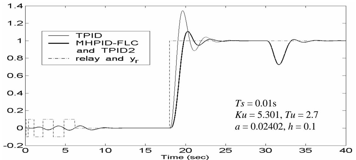
Figure 8.9 Comparison of set-point and load disturbance responses for  $G_3(s)$ .
