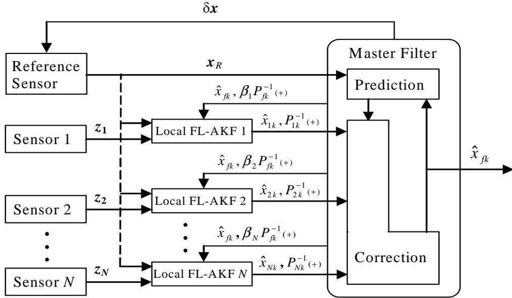
Figure 6.7 Fuzzy logic-based Adaptive Federated Kalman Filter (FL-AFKF).
