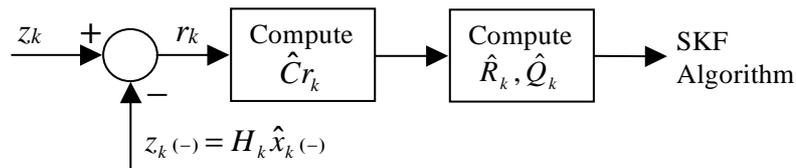
Figure 5.2 Additional blocks in the IAE filter.
