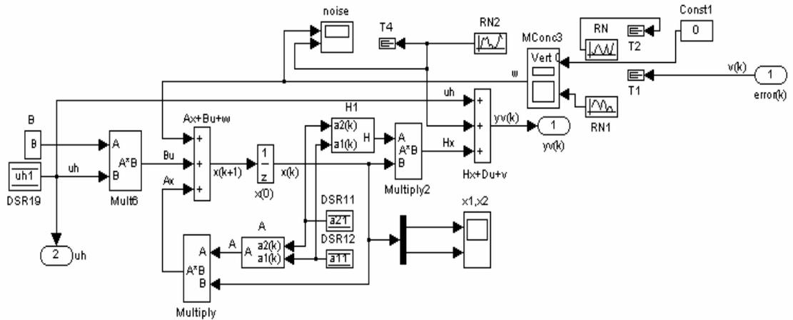
Figure B.25 Subsystem processmod: Neuro-Fuzzy-AKF, FL-AKF-FLA model.
