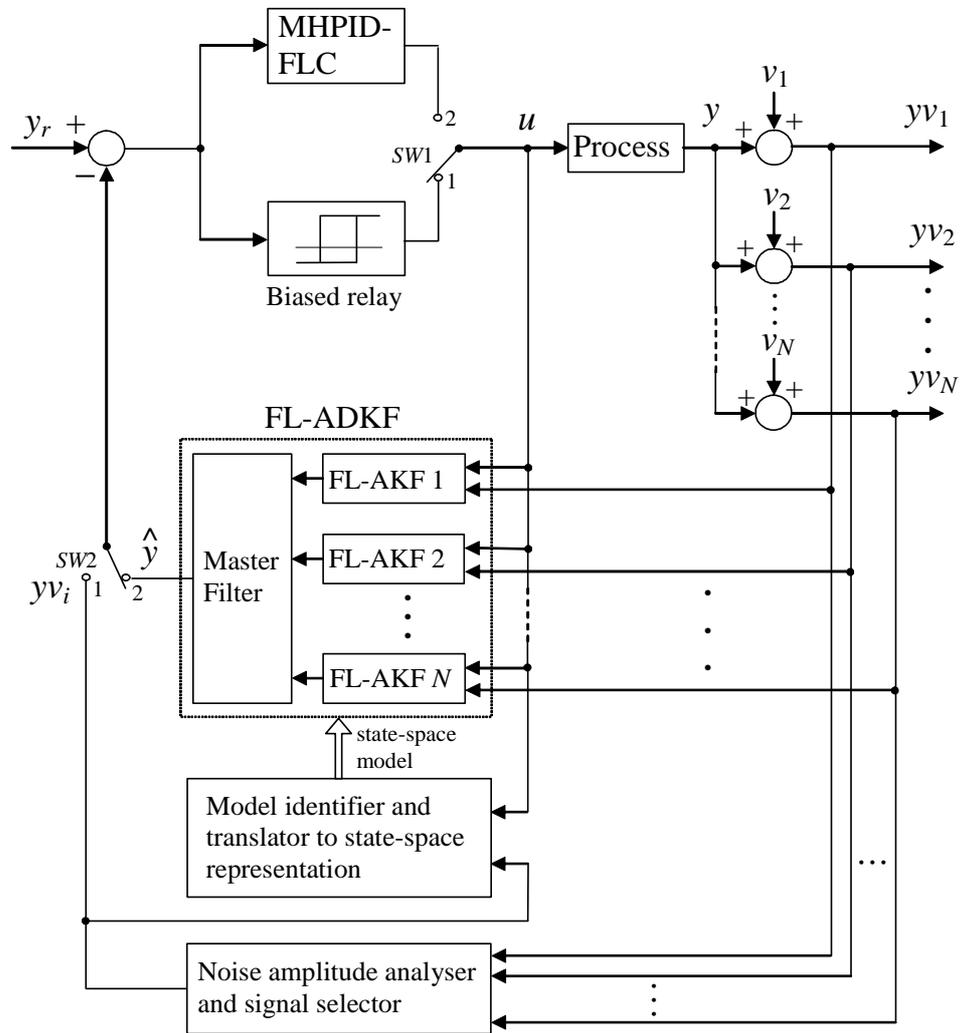
Figure 8.11 Auto-tuning the MHPID-FLC by using multiple noisy sensors.
