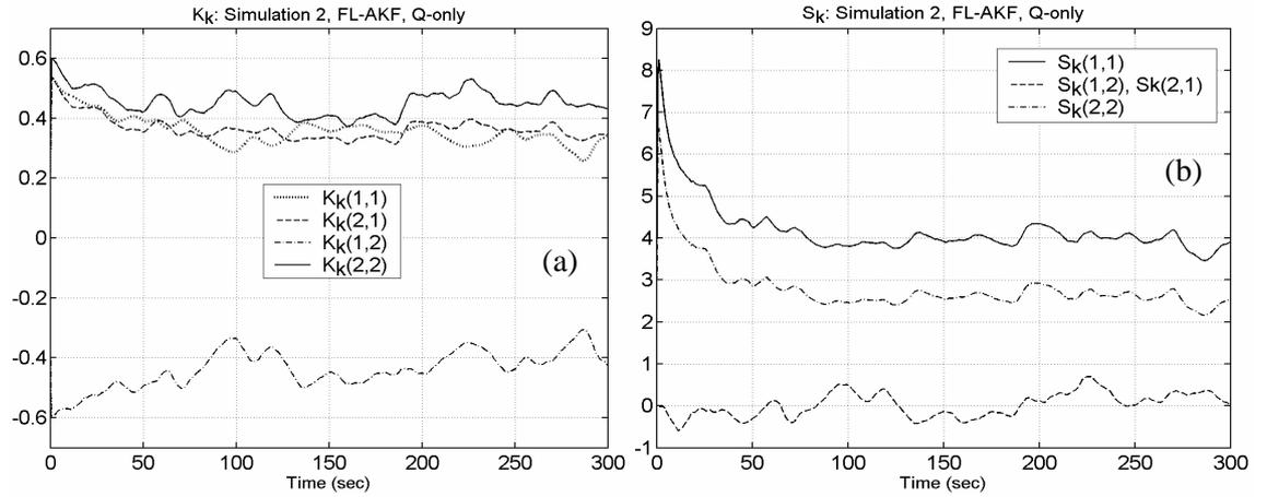
Figure 5.15(a) Elements of the Kalman gain matrix. (b) Elements of the residual covariance matrix; simulation 2, FL-AKF, Q-only case.
