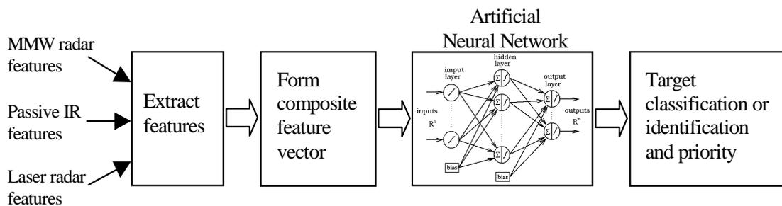
Figure 2.4 Feature-level fusion using an artificial neural network.
