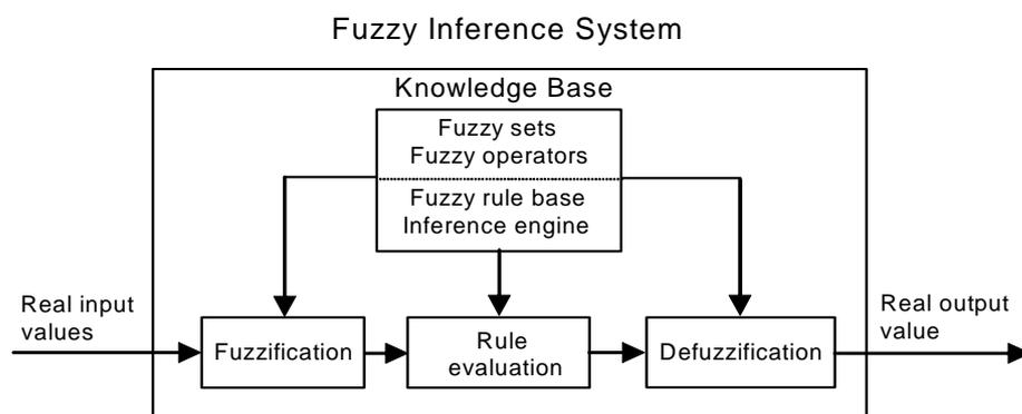
Figure 3.1 Basic structure of a FIS.
