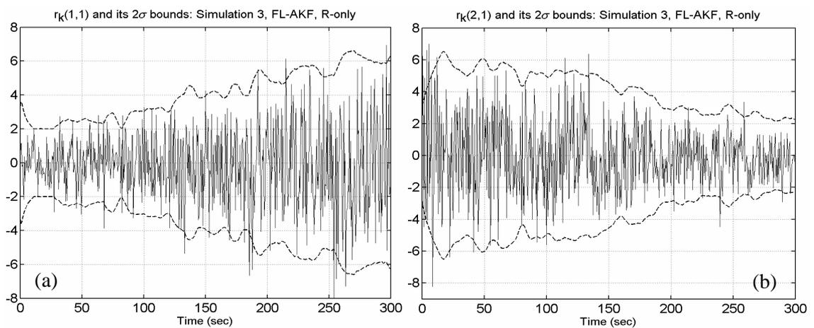
Figure 5.19 Residual sequences and their respective  $2\sigma$  bounds; Simulation 3, R-only case, non stationary measurement noise profiles used.
