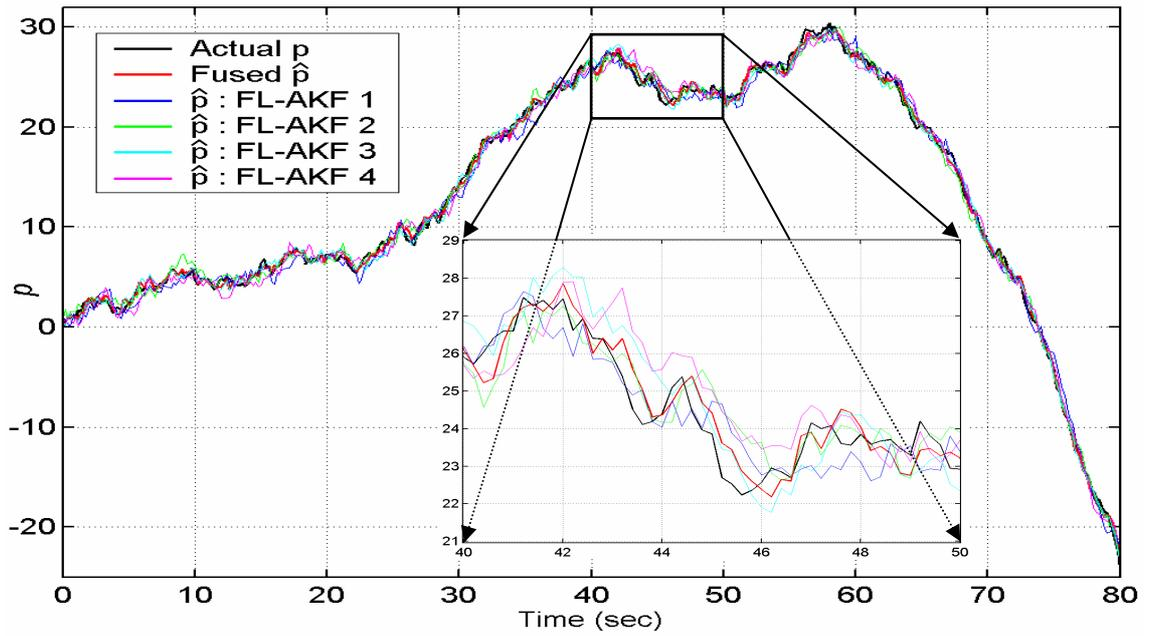
Figure 6.12 Actual position and estimated position of the vehicle obtained with the FL-ADKF and each of its local FL-AKFs, simulation 3.
