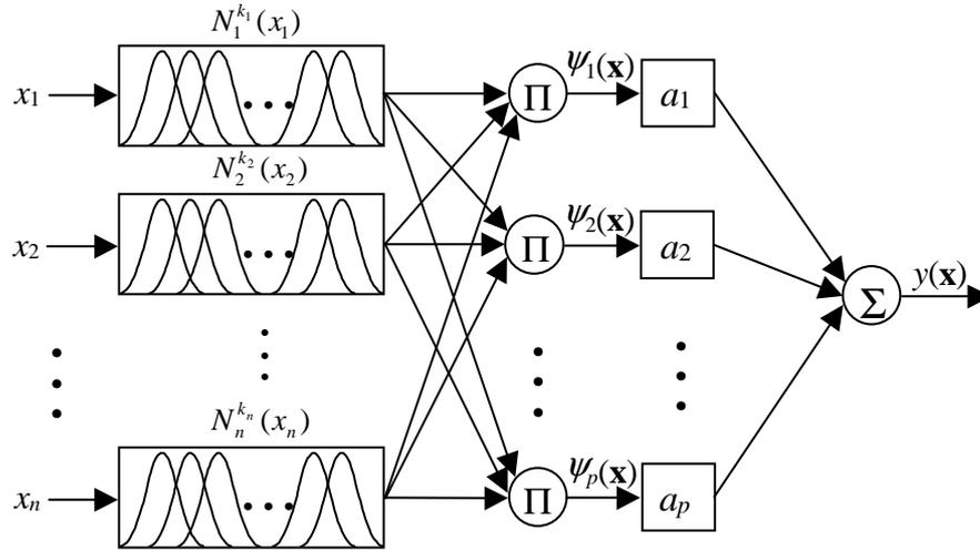
Figure 3.19 Structure of a neuro-fuzzy system using B-splines.
