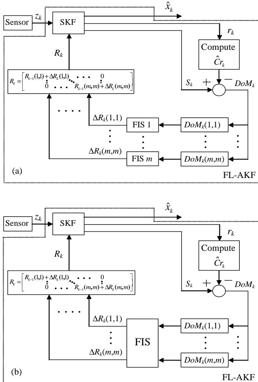
Figure 5.5 Graphical representations of the alternatives for implementing the algorithm to adjust  $R_k$ . (a)  $m$  parallel SISO FISs implementation. (b) MIMO FIS implementation.
