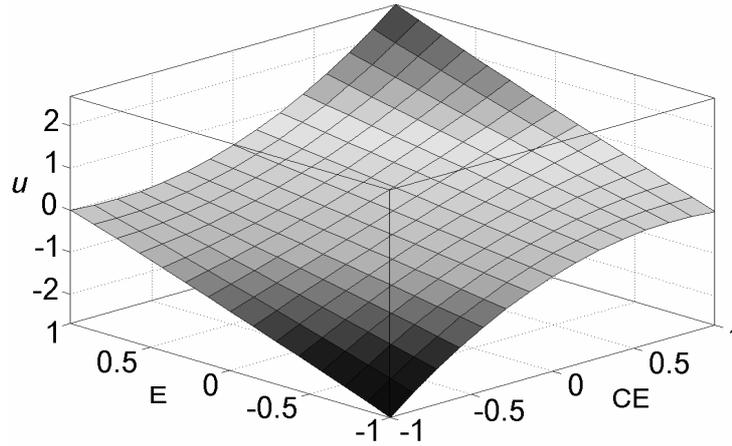
Figure 8.5 FCS control surface with modified consequent parameters.
