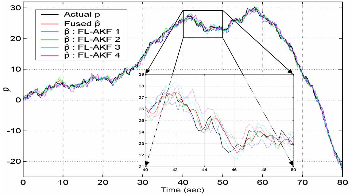
Figure 6.9 Actual position and estimated position of the vehicle obtained with the FL-AKF-FLA and each of its local FL-AKFs, simulation 1.
