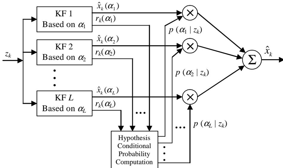
Figure 5.1 Structure of the MMAE filter.
