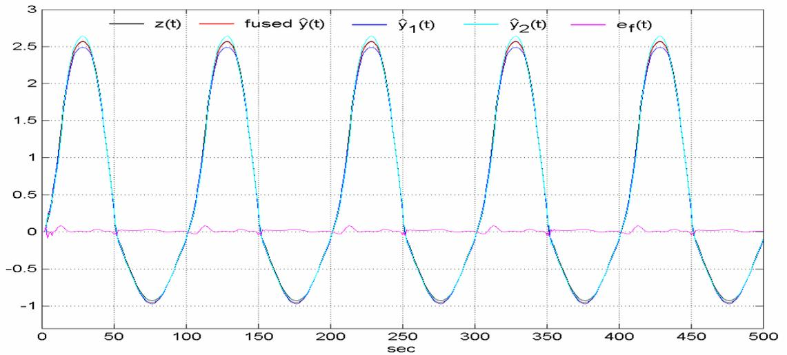
Figure 7.33 Fused and estimated signals compared with the actual noise free signal over the validation data.
