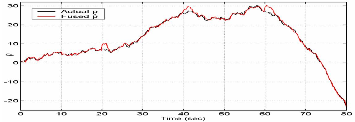
Figure 6.27 Actual position and estimated position of the vehicle obtained with the FL-ADKF, simulation 7.
