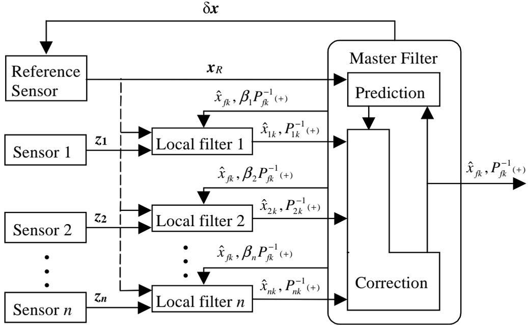
Figure 4.5 Federated Kalman filtering architecture.
