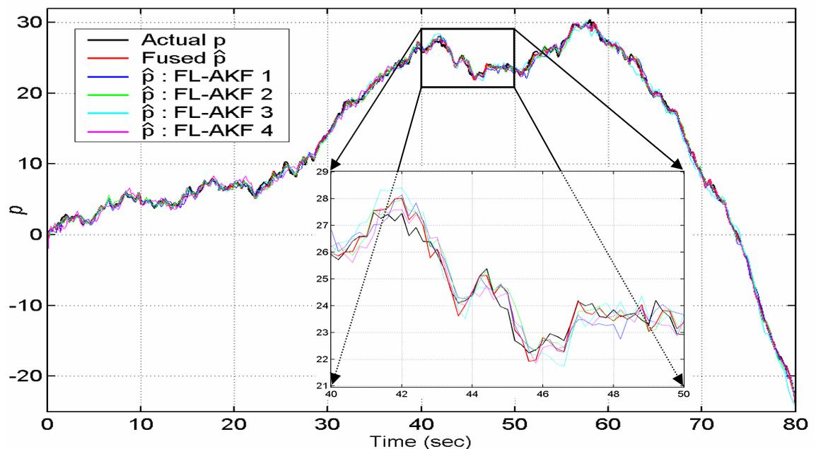
Figure 6.17 Actual position and estimated position of the vehicle obtained with the FL-ADKF and each of its local FL-AKFs, simulation 5.
