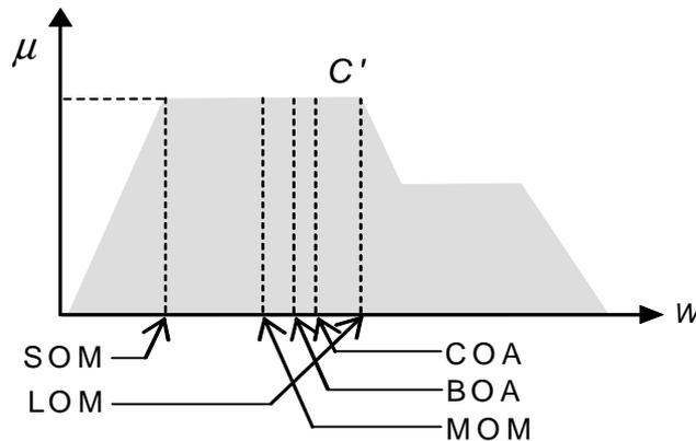
Figure 3.6 Comparison of the crisp FIS output obtained with the different defuzzification methods.
