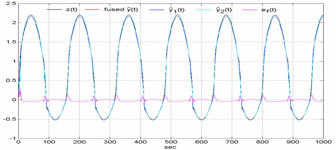
Figure 7.22 Fused and estimated signals compared with the actual noise free signal over the validation data.
