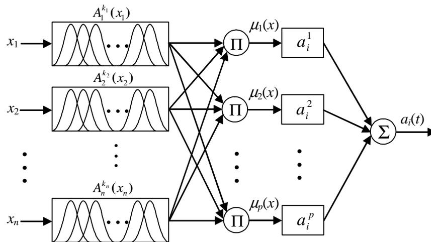
Figure 7.2 FIS used to approximate the parameters  $a_i(t)$ .
