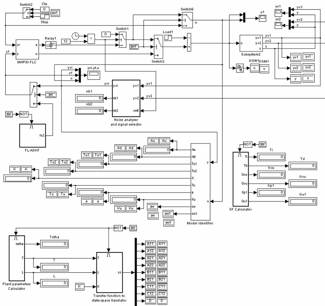
Figure B.29 The MHPID-FLC and MSDF model.
