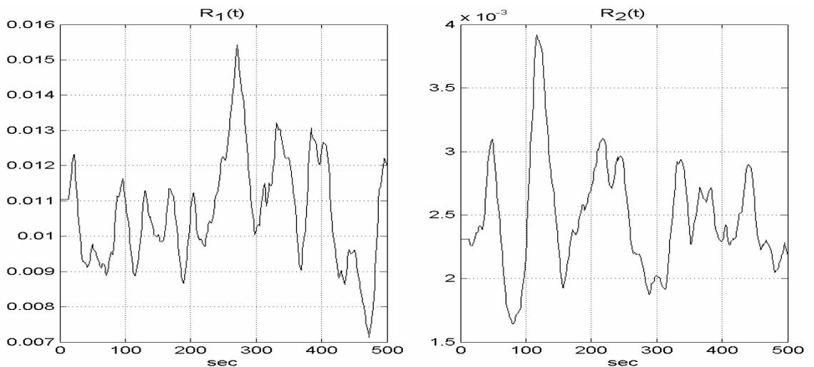
Figure 7.34 Measurement noise covariance values obtained during the validation process.
