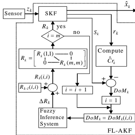
Figure 5.3 Graphical representation of the sequential algorithm to adjust  $R_k$  using a FIS.
