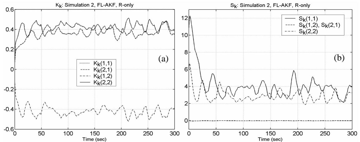
Figure 5.13(a) Elements of the Kalman gain matrix. (b) Elements of the residual covariance matrix; simulation 2, FL-AKF, R-only case.
