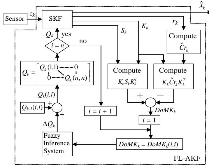
Figure 5.6 Graphical representation of the sequential algorithm to adjust  $Q_k$  using a FIS based on  $DoMK_k$ .
