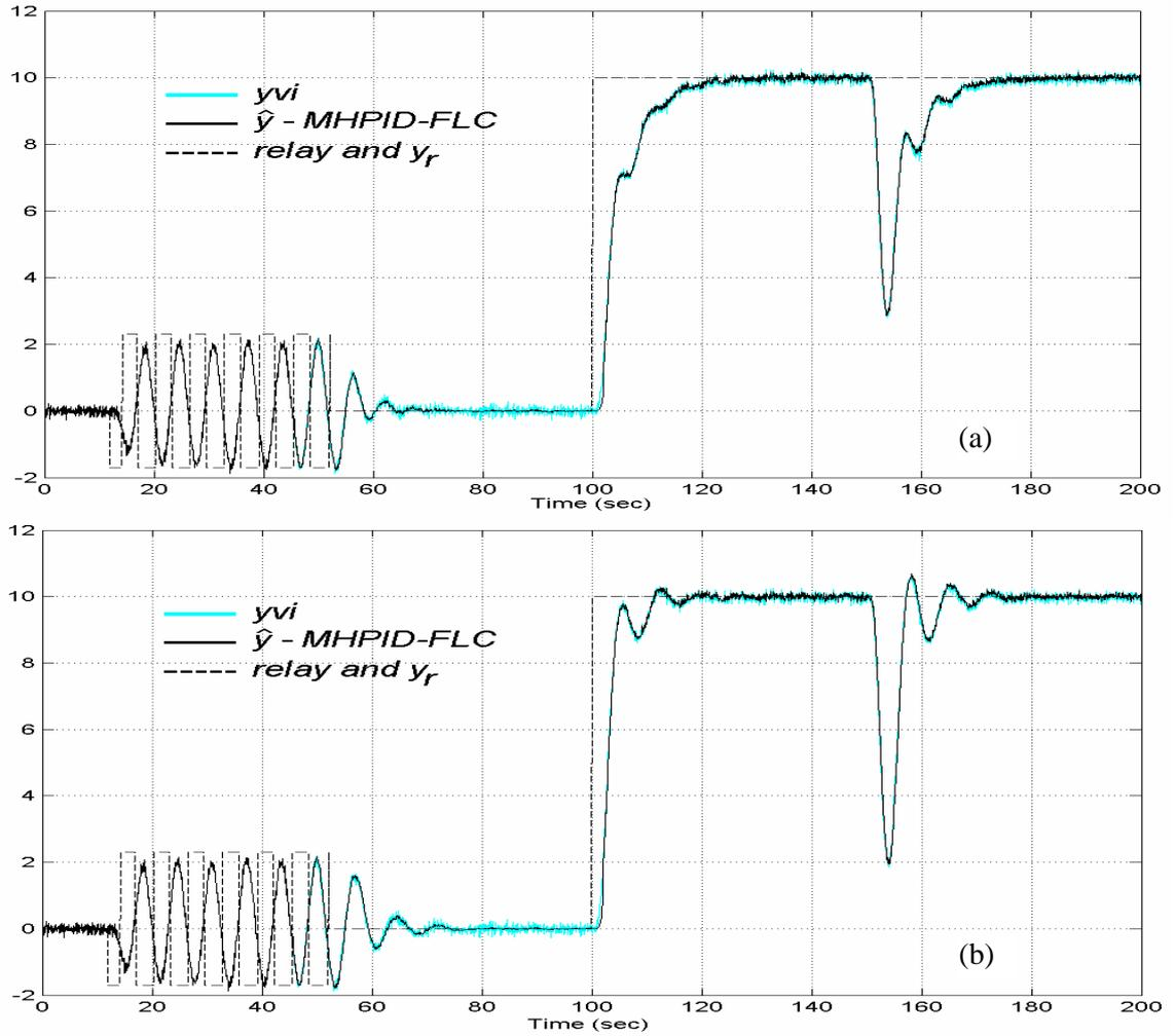
Figure 8.16 Set-point and load-disturbance responses for the plant in example 3, (a) with the original consequent parameters, (b) with the modified consequent parameters.
