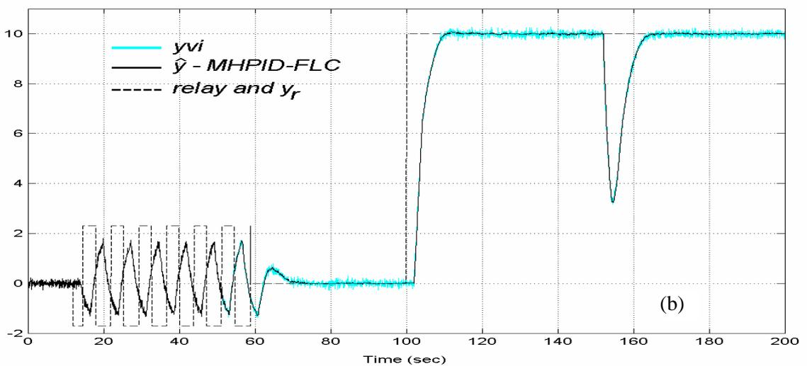
Figure 8.14 Set-point and load-disturbance responses for the plant in example 1, (a) with the original consequent parameters, (b) with the modified consequent parameters.
