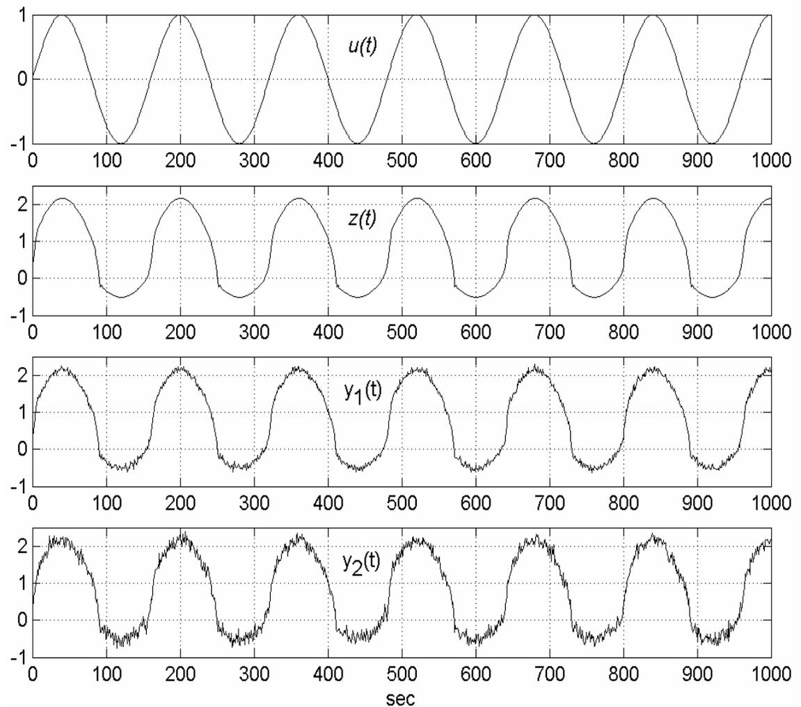
Figure 7.19 Validation signals generated with  $u(t)=\sin(\pi t/80)$ .
