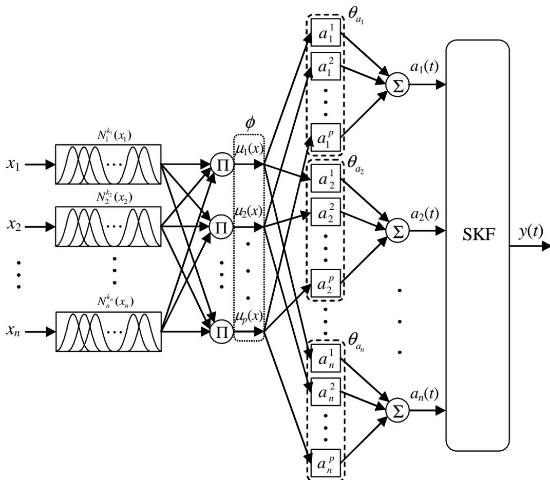
Figure 7.9 Connection between the simplified neuro-fuzzy network and a SKF.
