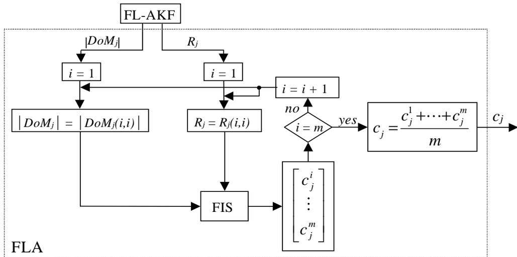
Figure 6.2 Process of calculating the degree of confidence values.
