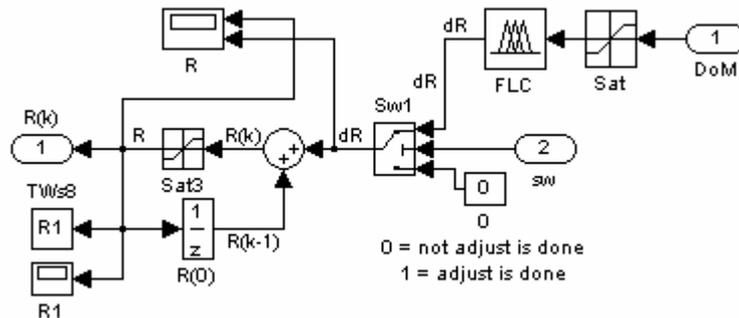
Figure B.27 Subsystem AdjustR: Neuro-Fuzzy-AKF, FL-AKF-FLA model.
