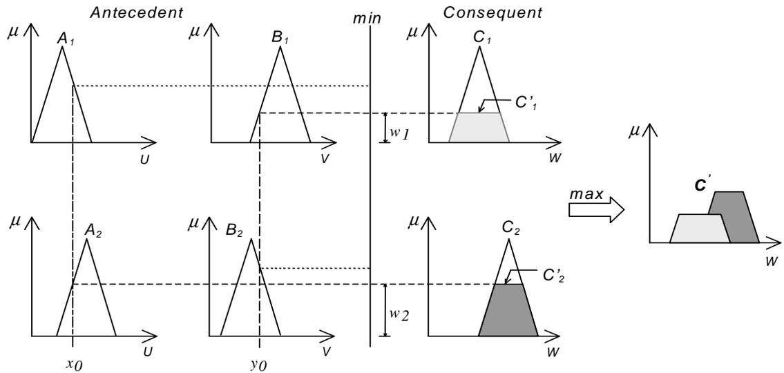
Figure 3.3 Graphical representation of the fuzzy reasoning procedure for multiple rules with multiple antecedents and *max-min compositional rule of inference* being used.
