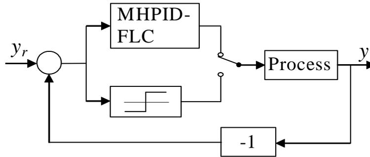
Figure 8.6 Relay feedback experiment.
