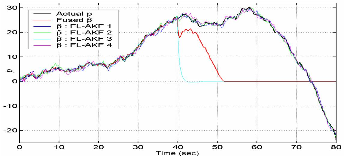
Figure 6.28 Actual and estimated position of the vehicle obtained with the FL-ADKF and each of its local FL-AKFs, simulation 8.
