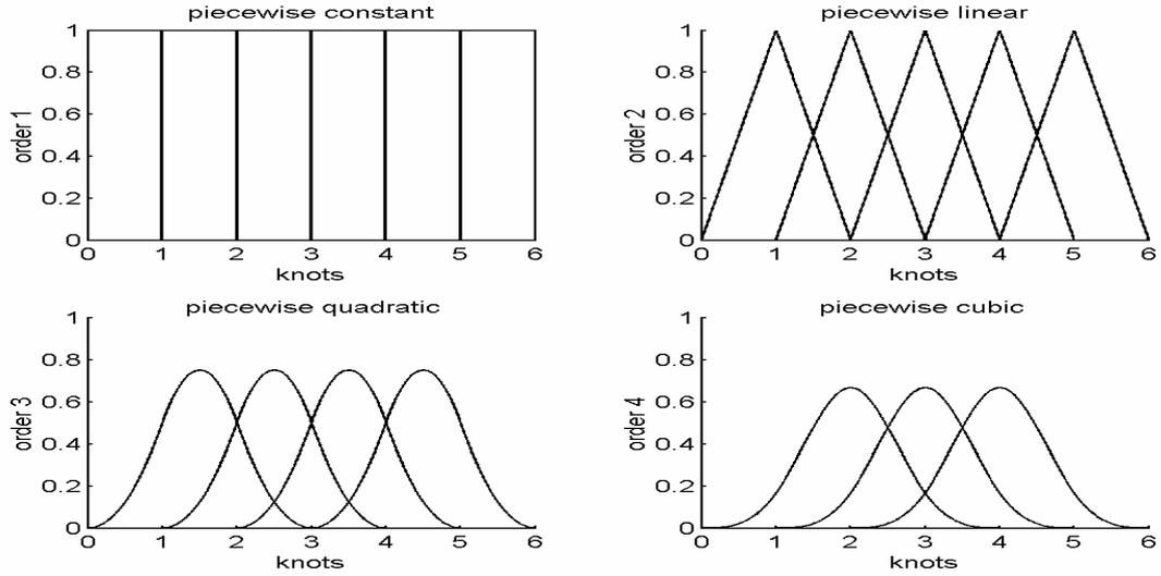
Figure 3.18 B-spline basis functions of order  $k = 1, 2, 3, 4$ , with knot vector  $= [0, 1, 2, 3, 4, 5, 6]^T$ .
