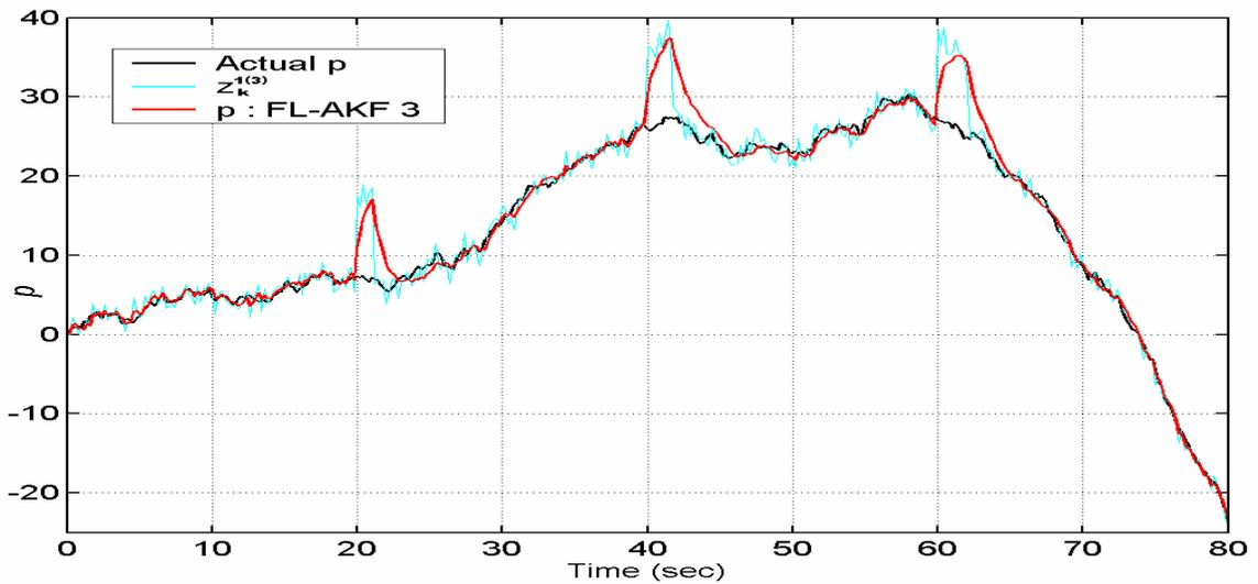
Figure 6.25 Actual position, measured position ( $z_k^{(3)}$ ), and estimated position of the vehicle obtained with the FL-AKF 3, FL-AKF-FLA, simulation 7.
