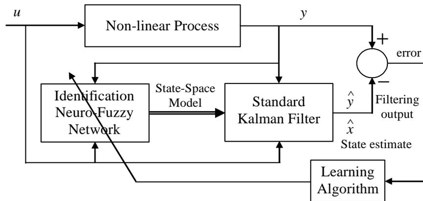
Figure 7.5 Direct neuro-fuzzy-SKF state estimation scheme.
