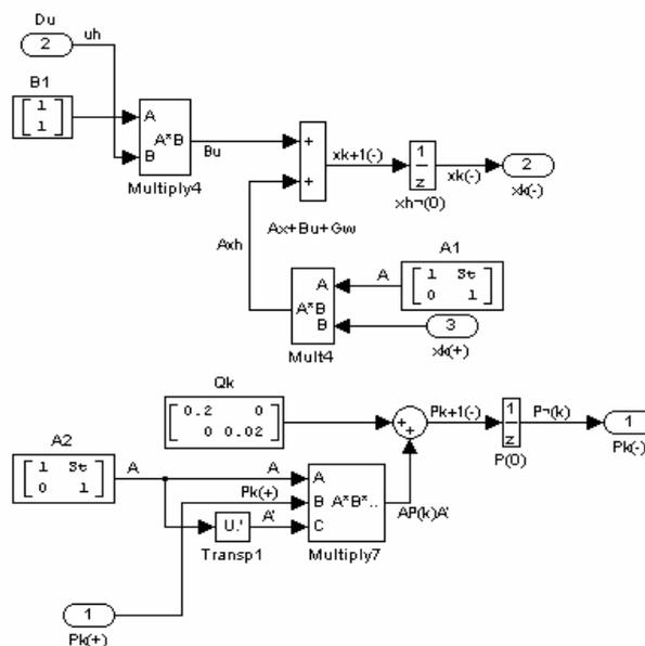
Figure B.15 Subsystem M-Filter: FL-ADKF model.
