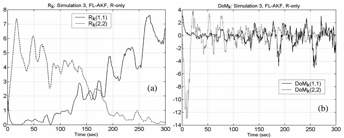
Figure 5.18(a) Diagonal estimated elements of matrix  $R_k$ . (b) Diagonal elements of matrix  $DoM_k$ ; Simulation 3, R-only case, non stationary measurement noise profiles used.
