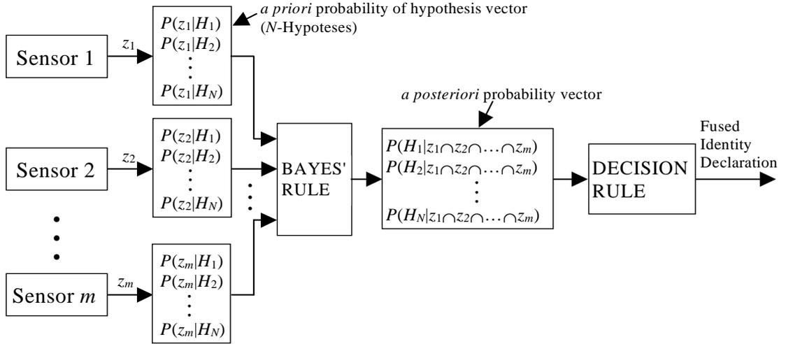
Figure 2.2 Graphical representation of an identity fusion process using Bayesian inference.
