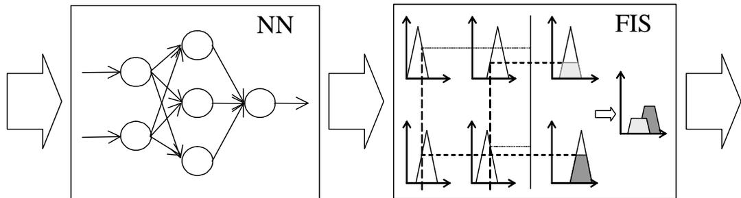
Figure 3.12 Concurrent neural/fuzzy system where a NN is used as pre-processor for a FIS.
