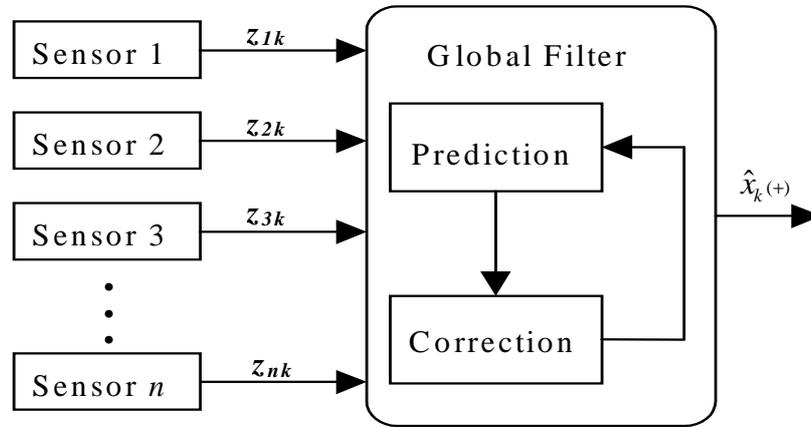
Figure 4.3 Centralised Kalman filtering architecture.
