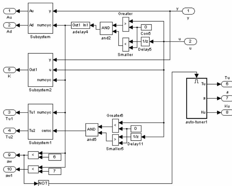
Figure B.31 Subsystem Model Identifier: MHPID-FLC and MSDF model.
