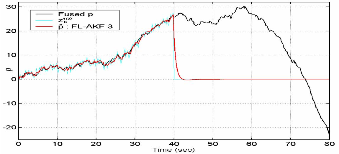
Figure 6.29 Actual position, measured position ( $z_k^{(3)}$ ), and estimated position of the vehicle obtained with the local FL-AKF 3, FL-ADKF, simulation 8.
