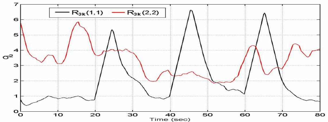
Figure 6.26 Adjustment of the elements in the main diagonal of matrix  $R_{3k}$ , FL-AKF 3, FL-AKF-FLA, simulation 7.
