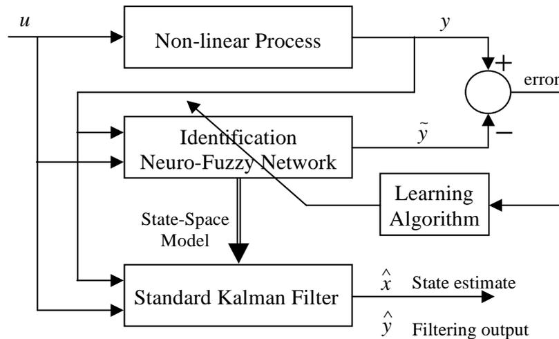
Figure 7.4 Indirect neuro-fuzzy-SKF state estimation scheme.
