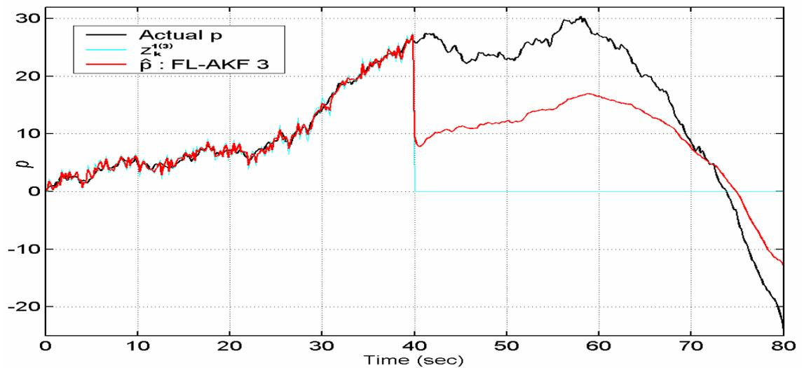
Figure 6.33 Actual position, measured position ( $z_k^{(a)}$ ), and estimated position of the vehicle obtained with the FL-AKF 3, FL-AFKF, simulation 8.
