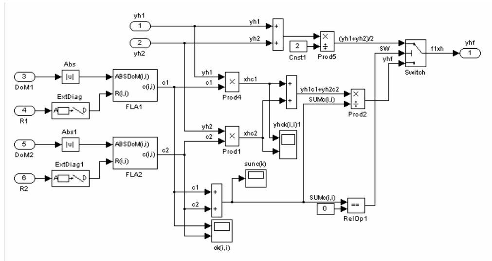
Figure B.28 Subsystem FUSION: Neuro-Fuzzy-AKF, FL-AKF-FLA model.
