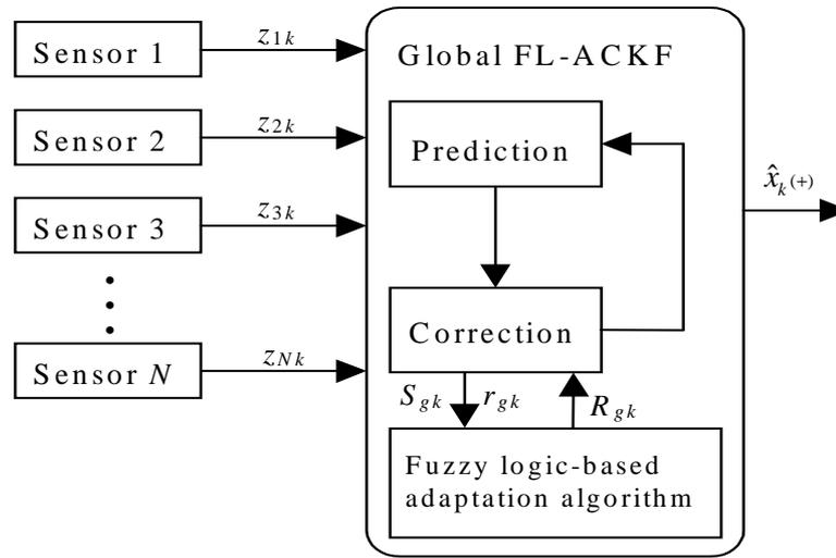
Figure 6.4 Fuzzy logic-based Adaptive Centralised Kalman Filter (FL-ACKF).
