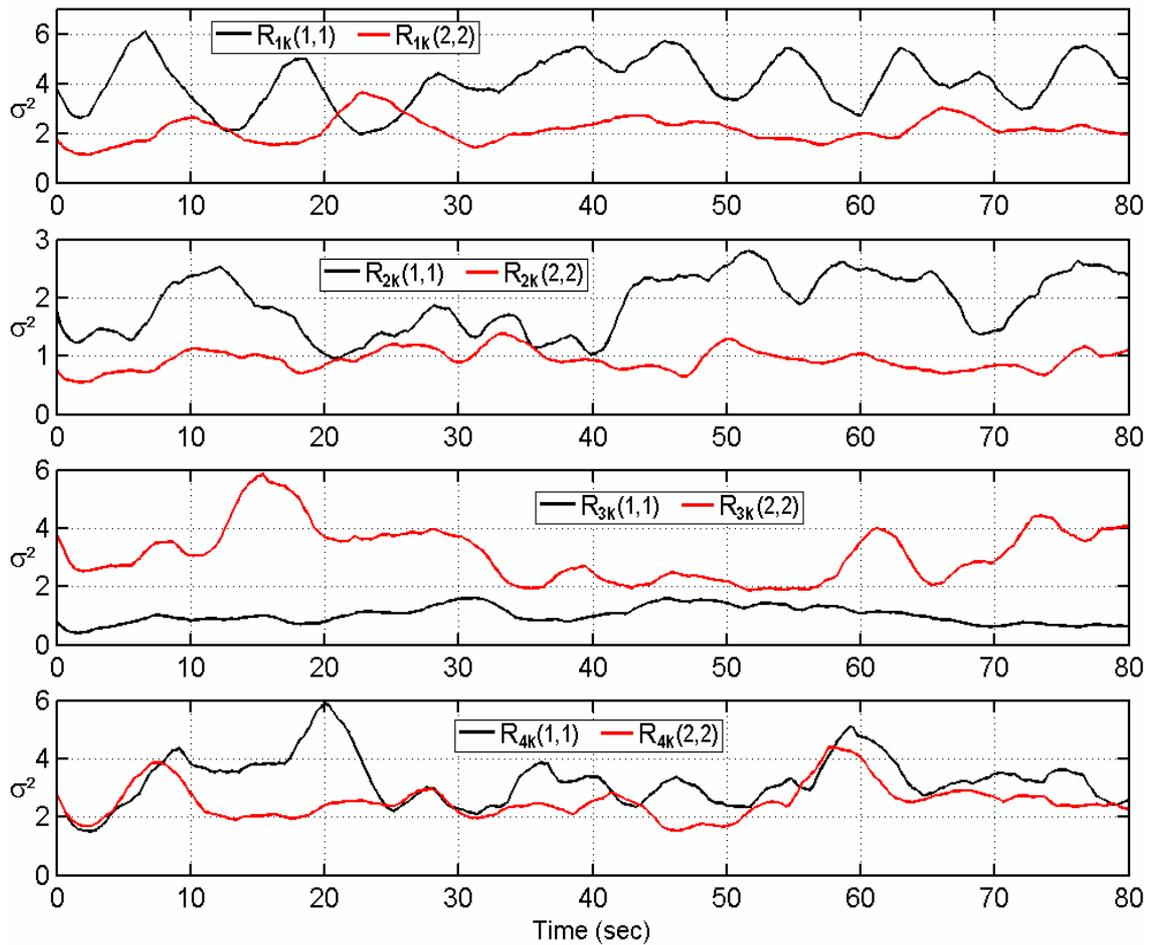
Figure 6.13 Adjustment of the elements in the main diagonal of matrices  $R_{1k}$ ,  $R_{2k}$ ,  $R_{3k}$ , and  $R_{4k}$  in each of the local FL-AKFs of the FL-ADKF, Simulation 3.
