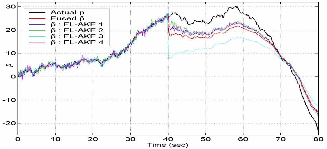
Figure 6.32 Actual and estimated position of the vehicle obtained with the FL-AFKF and each of its local FL-AKFs, simulation 8.
