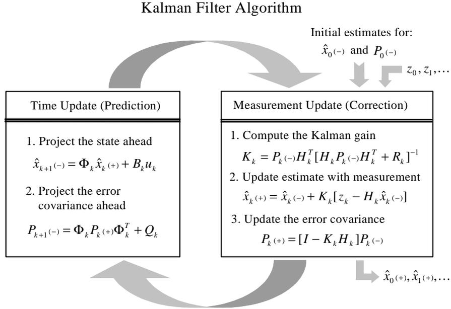
Figure 4.1 Graphical representation of the Kalman filter algorithm.
