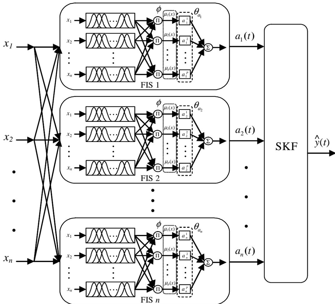
Figure 7.6 Connection between the neuro-fuzzy network of figure 7.3 and a SKF.
