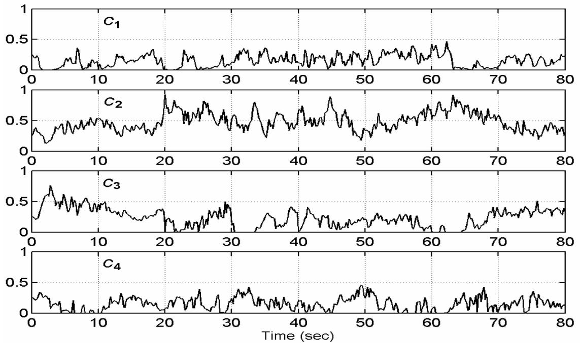
Figure 6.22 Degree of confidence factors assigned to each local FL-AKF state-vector estimate in the FL-AKF-FLA approach, simulation 6.
