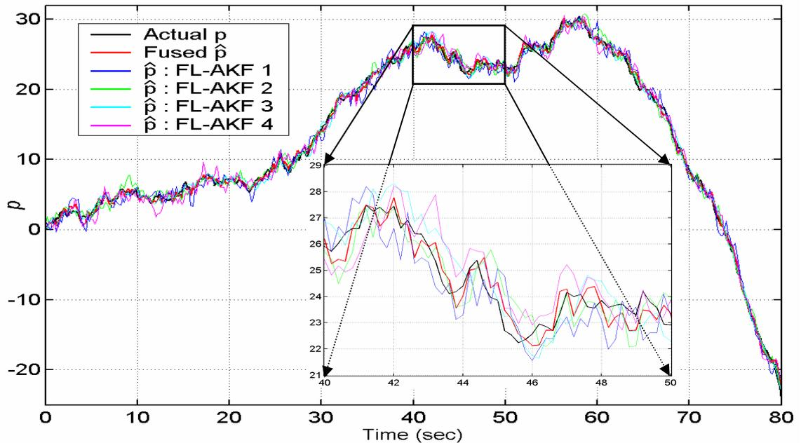
Figure 6.11 Actual position and estimated position of the vehicle obtained with the FL-ADKF and each of its local FL-AKFs, simulation 2.
