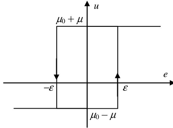
Figure 8.12 The biased relay.
