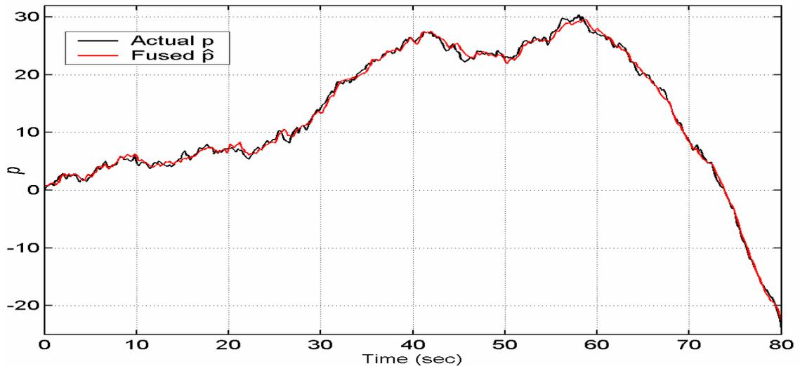
Figure 6.19 Actual position and estimated position of the vehicle obtained with the FL-AKF-FLA architecture, simulation 6.
