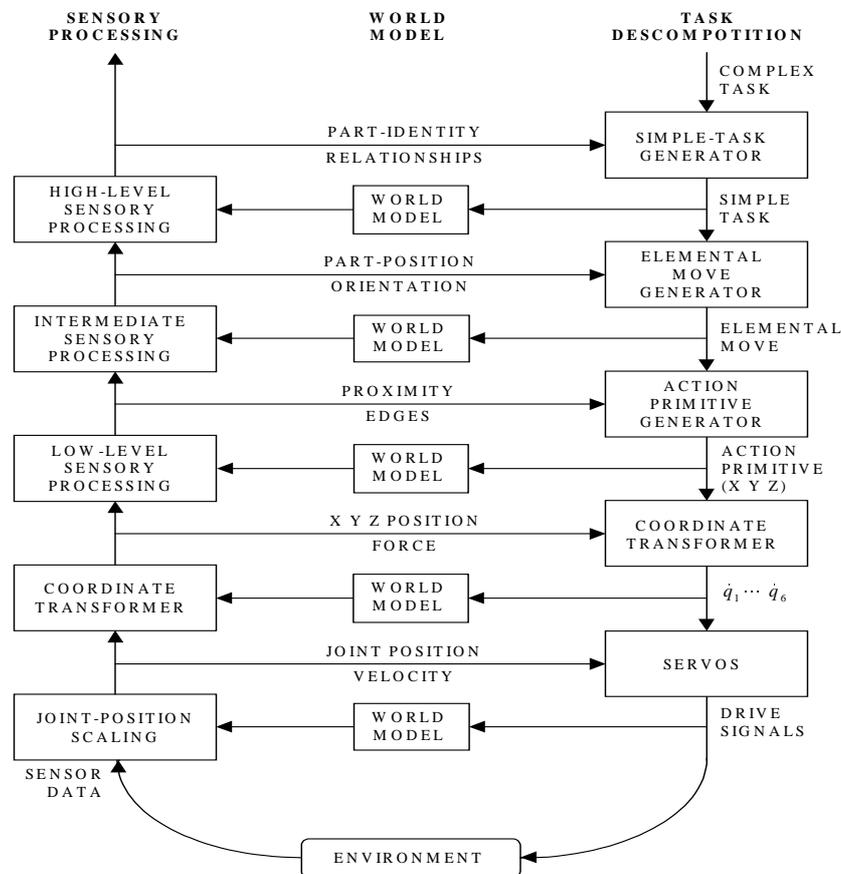
Figure 1.1 NBS sensory and control hierarchy used to control a multi-sensory robot (adapted from [Luo and Kay, 1989]).
