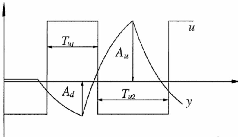
Figure 8.13 Oscillatory waveforms under a biased relay feedback (adapted from [Wang *et al*, 1997]).
