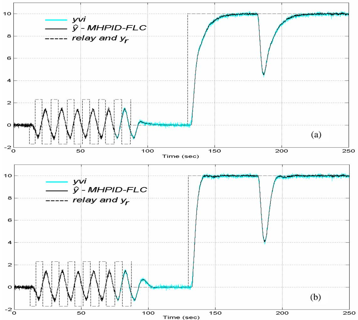
Figure 8.15 Set-point and load-disturbance responses for the plant in example 2, (a) with the original consequent parameters, (b) with the modified consequent parameters.
