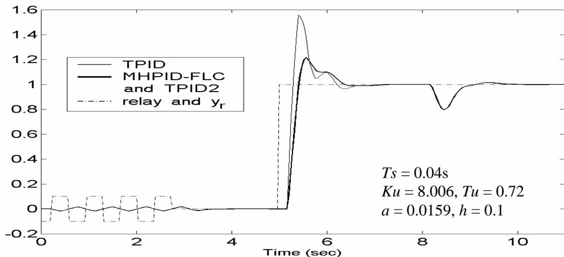
Figure 8.7 Comparison of set-point and load disturbance responses for  $G_1(s)$ .
