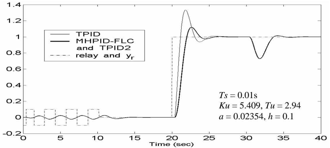
Figure 8.8 Comparison of set-point and load disturbance responses for  $G_2(s)$ .
