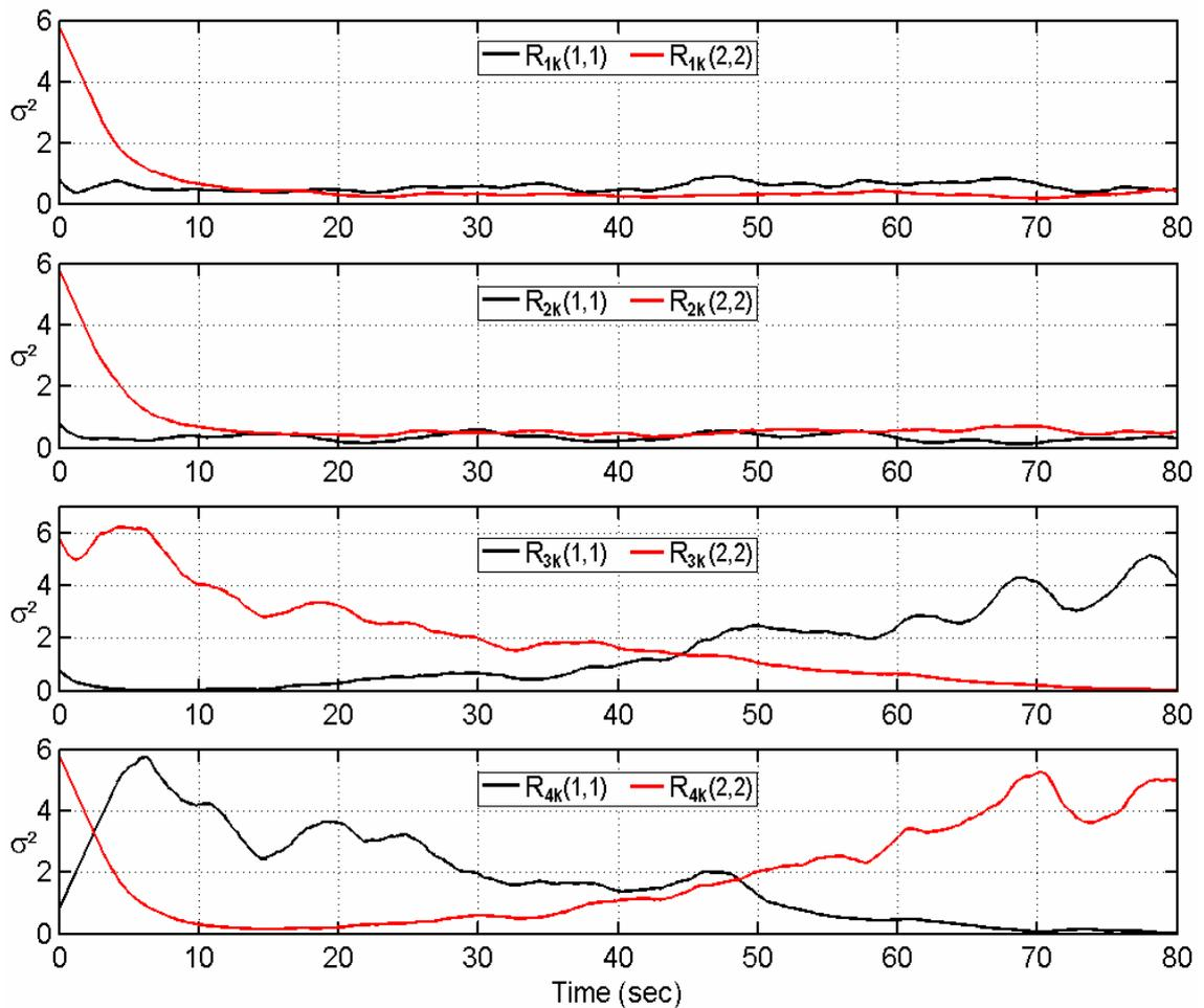
Figure 6.18 Adjustment of the elements in the main diagonal of matrices  $R_{1k}$ ,  $R_{2k}$ ,  $R_{3k}$ , and  $R_{4k}$  in each of the local FL-AKFs of the FL-ADKF, simulation 5.
