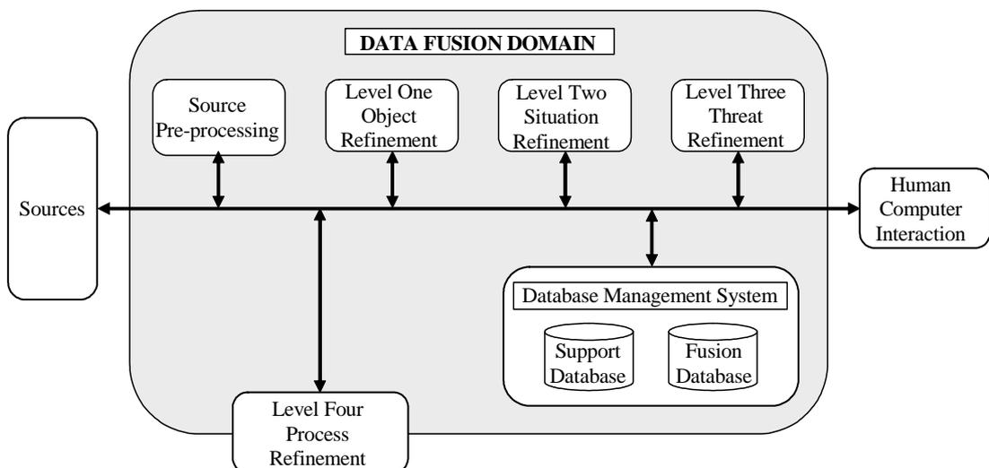
Figure 1.2 Basic components of the JDL data fusion process model (adapted from [Hall, 2002]).
