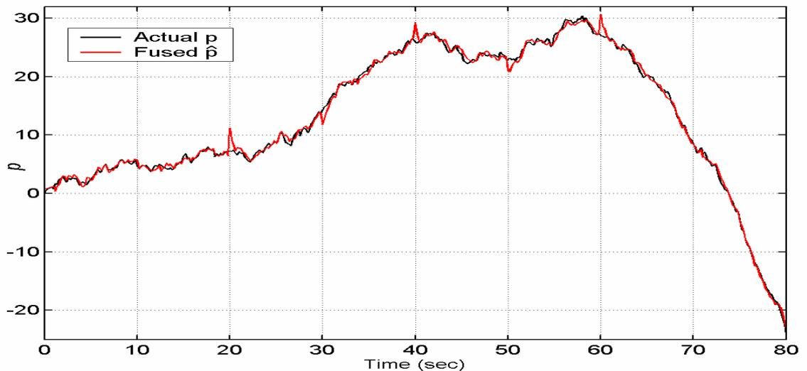
Figure 6.23 Actual position and estimated position of the vehicle obtained with the FL-ADKF, simulation 6.
