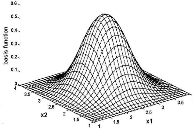
Figure 3.20 A two-dimensional quadratic multivariable B-spline basis function.
