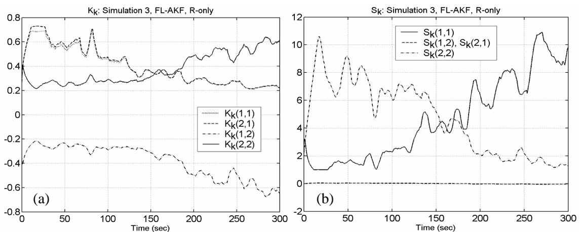
Figure 5.20(a) Elements of the Kalman gain matrix. (b) Elements of the residual covariance matrix; Simulation 3, R-only case, non stationary measurement noise profiles used.
