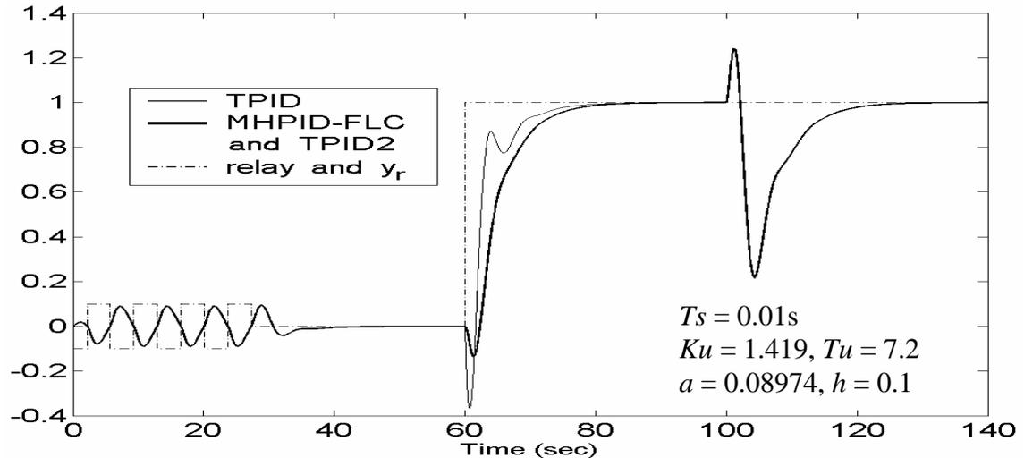
Figure 8.10 Comparison of set-point and load disturbance responses for  $G_4(s)$ .
