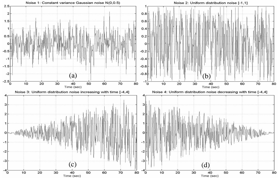
Figure 6.16 Noise profiles used in simulation 5; (a) Constant variance Gaussian noise sequence  $N(0,0.5)$ ; (b) Uniform distribution random noise sequence  $[-1,1]$ ; (c) Uniform distribution random noise sequence increasing with time  $[-4,4]$ ; (d) Uniform distribution random noise sequence decreasing with time  $[-4,4]$ .
