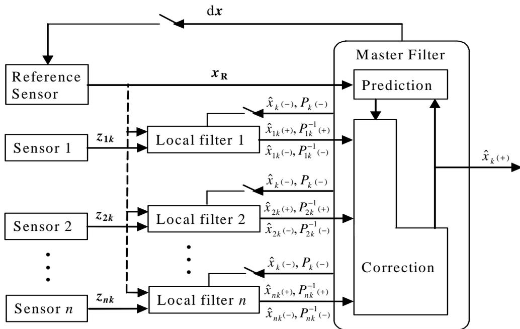
Figure 4.4 Decentralised Kalman filtering architecture.
