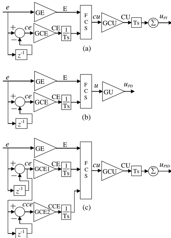
Figure 8.1 Structures for (a) PI-FLC, (b) PD-FLC, and (c) PID-FLC.
