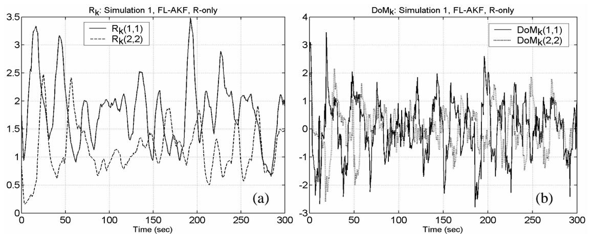
Figure 5.10(a) Estimated diagonal elements of the measurement noise covariance matrix  $R_k$ . (b) Diagonal elements of matrix  $DoM_k$ ; simulation 1, FL-AKF, R-only case.
