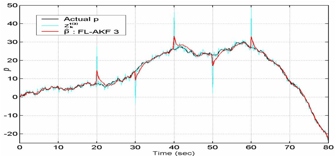
Figure 6.20 Actual position, measured position ( $z_k^{(3)}$ ), and estimated position of the vehicle obtained with the FL-AKF 3, FL-AKF-FLA, simulation 6.
