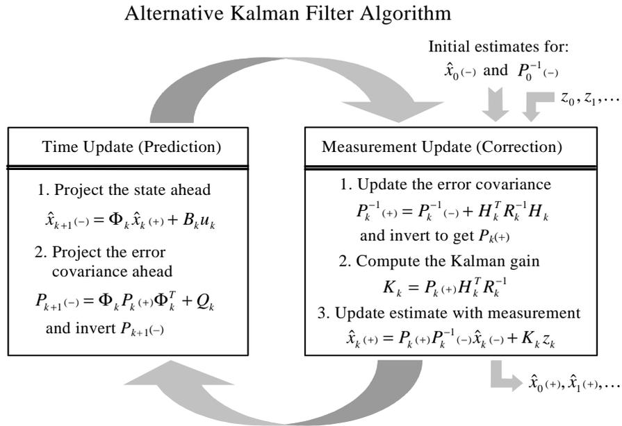
Figure 4.2 Graphical representation of the alternative Kalman filter algorithm.
